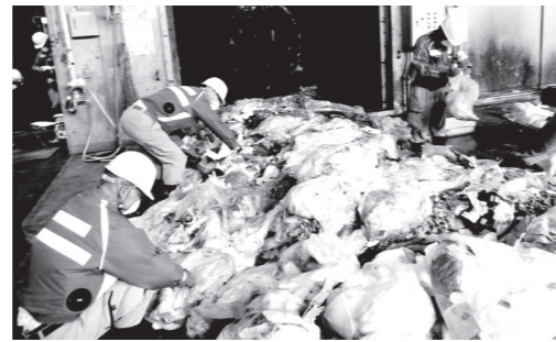
Inspection on incoming waste (Nerima Incineration Plant)
